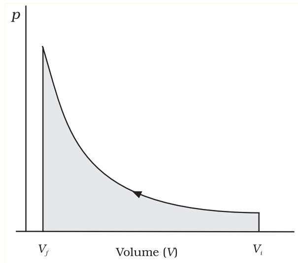
**Fig. 6.5 (c)**  $pV$ -plot when pressure is not constant and changes in infinite steps (reversible conditions) during compression from initial volume,  $V_i$  to final volume,  $V_f$ . Work done on the gas is represented by the shaded area.
