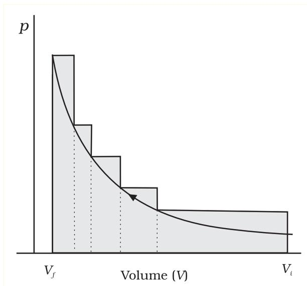
**Fig. 6.5 (b)**  $pV$ -plot when pressure is not constant and changes in finite steps during compression from initial volume,  $V_i$  to final volume,  $V_f$ . Work done on the gas is represented by the shaded area.
