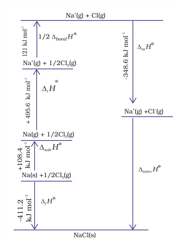
**Fig. 6.9** Enthalpy diagram for lattice enthalpy of NaCl
