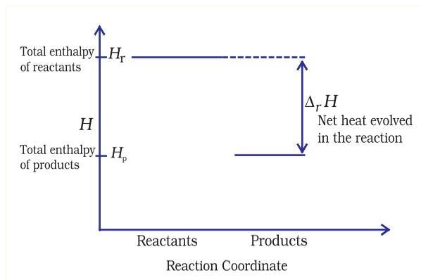
**Fig. 6.10 (a)** Enthalpy diagram for exothermic reactions
