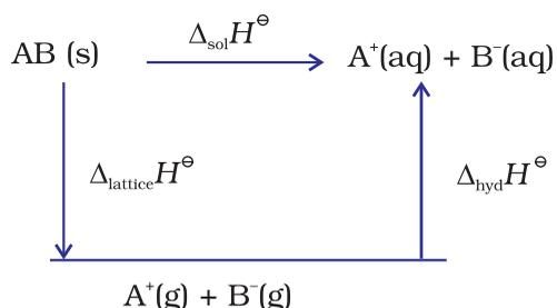
The enthalpy of solution of AB(s),  $\Delta_{\text{sol}} H^\ominus$ , in water is, therefore, determined by the selective values of the lattice enthalpy,  $\Delta_{\text{lattice}} H^\ominus$  and enthalpy of hydration of ions,  $\Delta_{\text{hyd}} H^\ominus$  as
