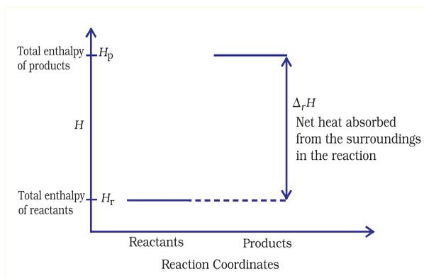
**Fig. 6.10 (b)** Enthalpy diagram for endothermic reactions
